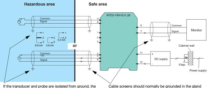
If the transducer and probe are isolated from ground, the cable screen may be left unconnected at this end but must be securely insulated. If the transducer circuitry is connected or decoupled to ground the screen must be securely grounded.
